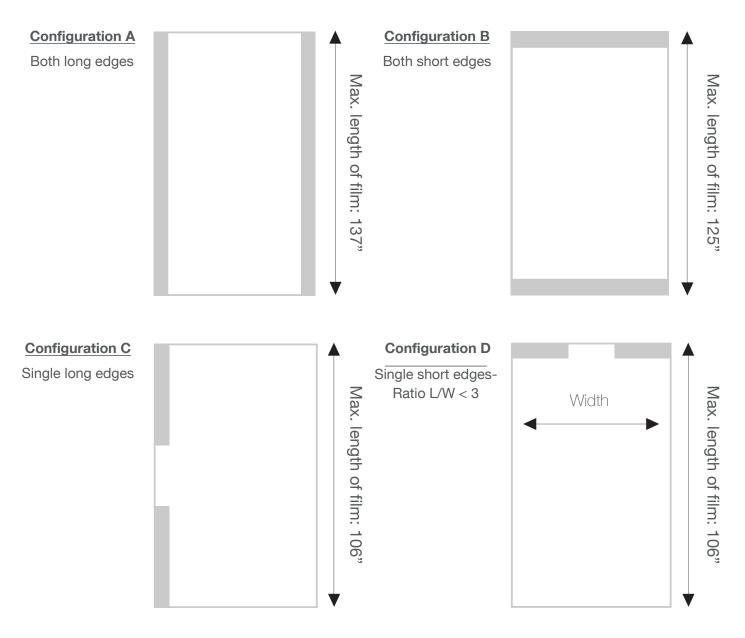
The technical note defines the different options for busbar location and the respective limitations with respect to Decorative Film switch film length. Any configuration other than what is shown here will require Decorative Films' technical approval.
